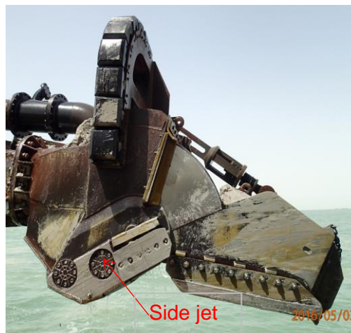
Figure 3.2 Draghead with side jetting nozzle
