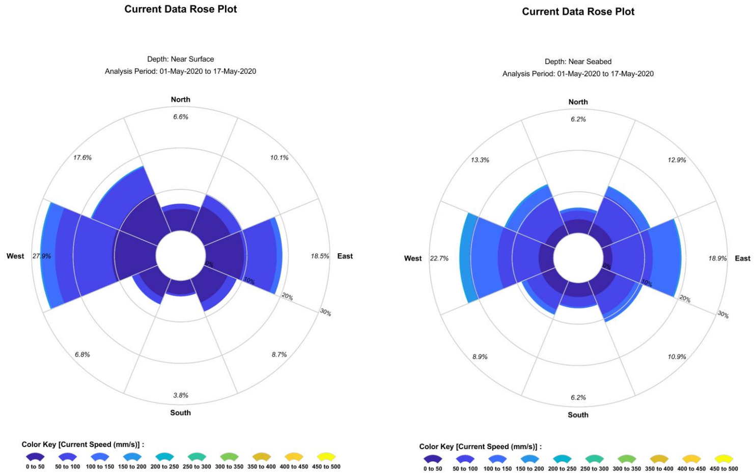
Figure 5 Near-surface and near-seabed current speed and direction at SG2a (Watchkeeper) during May 2020. Speed intervals of 50 mm/s are used.
