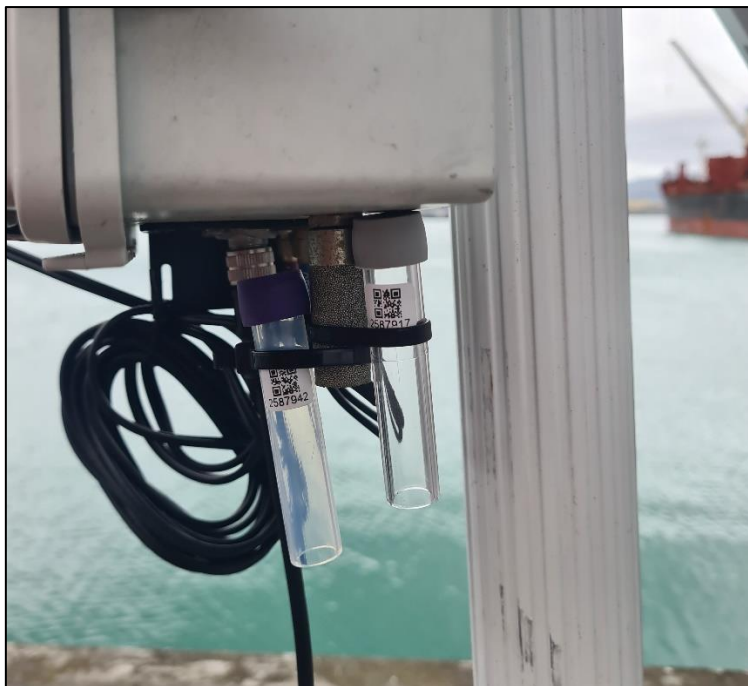
Figure 5: Nitrogen dioxide and sulphur dioxide diffusion tubes (with QR codes) mounted underneath the PM 2.5 monitor at the end of the LPC tug boat wharf at the Port. ( Image taken on 26 March 2025 )
